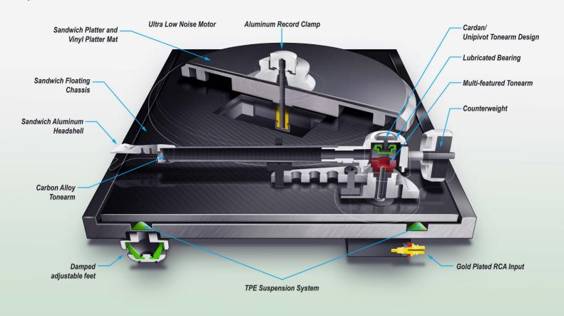
Aluminum Record Clamp precision machined heavy aluminum for added mass, damping, and lower distortion. Creates a more secure and precise coupling for vinyl stability during playback.
